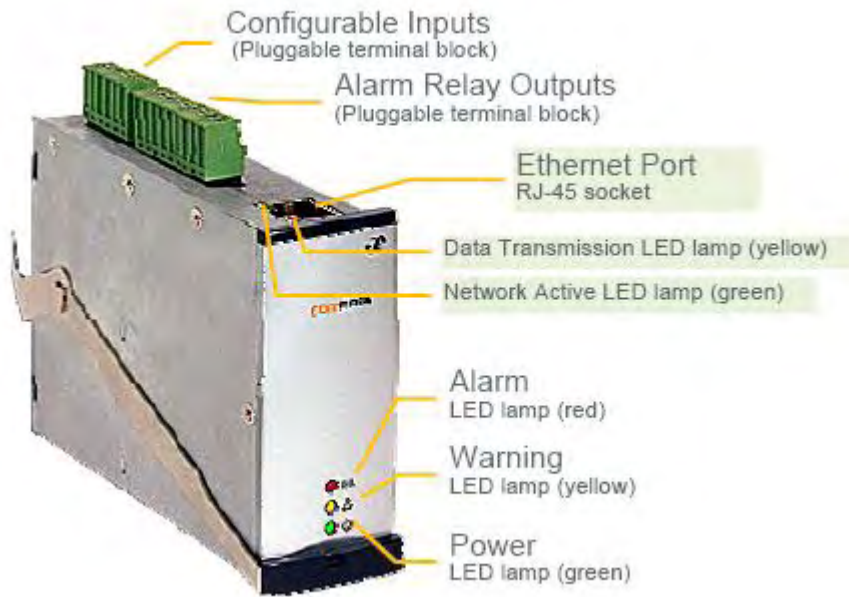
Figure 3 Location of I/O terminals, Ethernet port and LED lamps.
