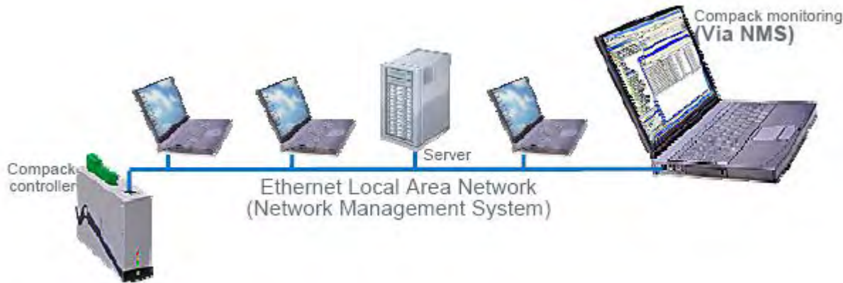
Figure 13 Power system remote monitoring via NMS.
