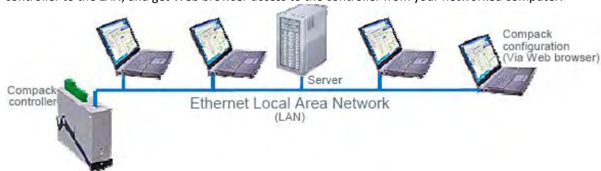
Figure 8 Controller’s access from a computer connected a LAN
