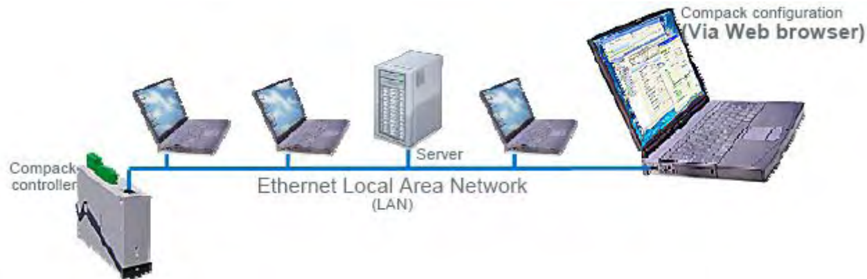
Figure 11 Power system configuration via Web browser.
